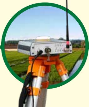
RTK GPS base station with integrated GPS antenna and radio modem.
