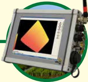
Board computer with 8,4" touchscreen display and integrated GPS RTK rover. This solution: reduces wiring, makes it easier to move it to different tractors and allows to graphically display earthworks.
